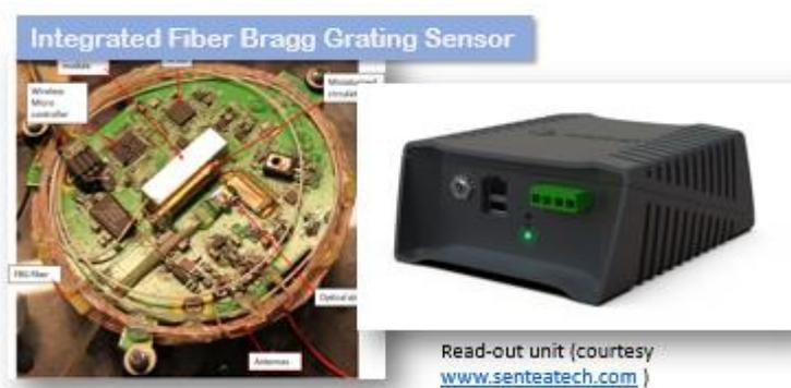
Fiber Bragg Grating (FBG) sensors are widely used in applications requiring multi-point strain or temperature sensing, e.g. in structural health monitoring of bridges, dams and buildings. Also, increasing the efficiency of wind turbines and monitoring chemical processes are important applications. They can operate in harsh environments and are immune to electromagnetic radiation.
