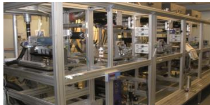
ROKO – in-air roll-to-roll pilot line
